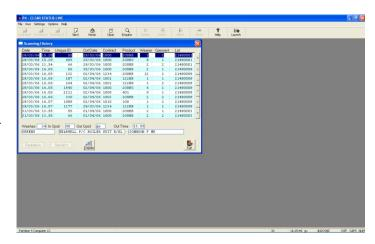
The screen (above) shows the display for a selected garment (66) and displays the dates of each process the garment has had. This information is stored on line for as long as required and can be archived on to long-term storage to provide the ultimate degree of traceability.
